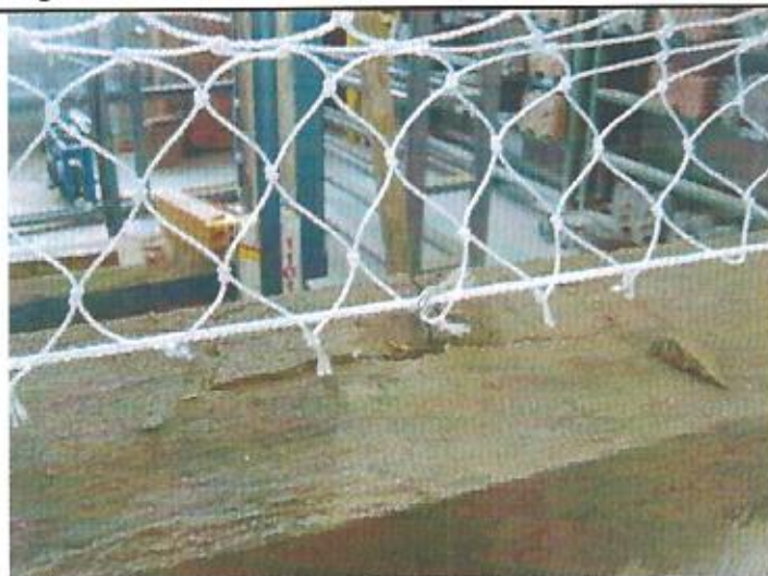
Fig. 2 – Details of hook and anchor slippage at the central bottom part of frame
